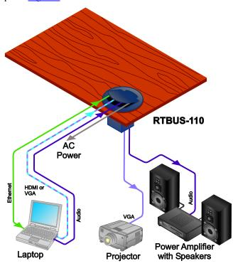
Figure 4: RTBUS-110 Boardroom Installation
